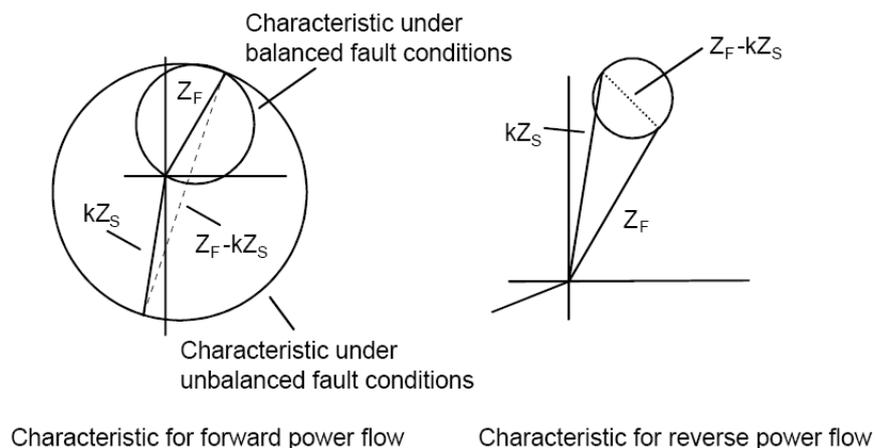
Figure 1, Cross-Polarised Mho Characteristic
