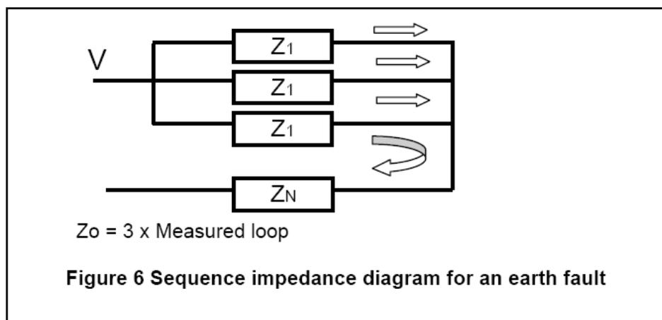
Figure 6 shows the method utilised to measure the zero sequence impedance of a line that gives the expression.;
