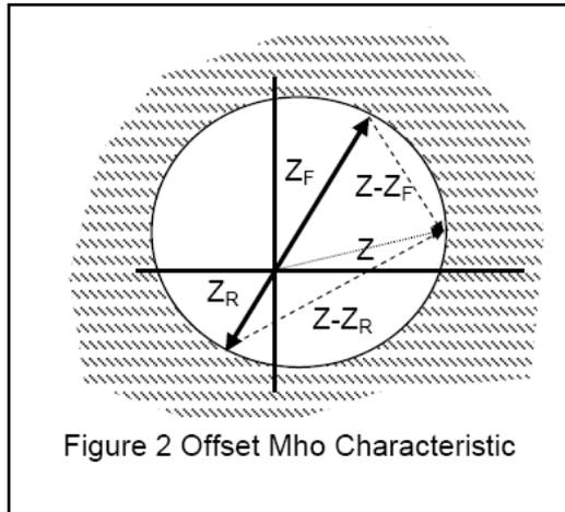
The offset Mho characteristic is shown in figure 2. The characteristic is set with a forward reach,  $Z_F$  and a reverse reach,  $Z_R$ . This type of characteristic may be selected for Zone 3, and it provides time delayed back-up for faults behind the relaying point.
