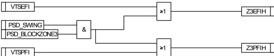
Zone 4 does have memory voltage, so inhibit from all, ie Power Swing, VTS, or Vmem timed out.
