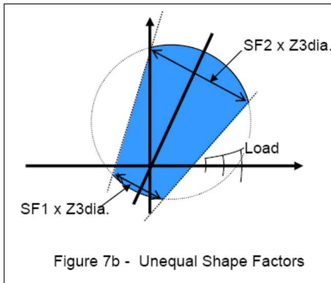
The above figure shows the position of blinders if different values are chosen for SF1 & SF2.
