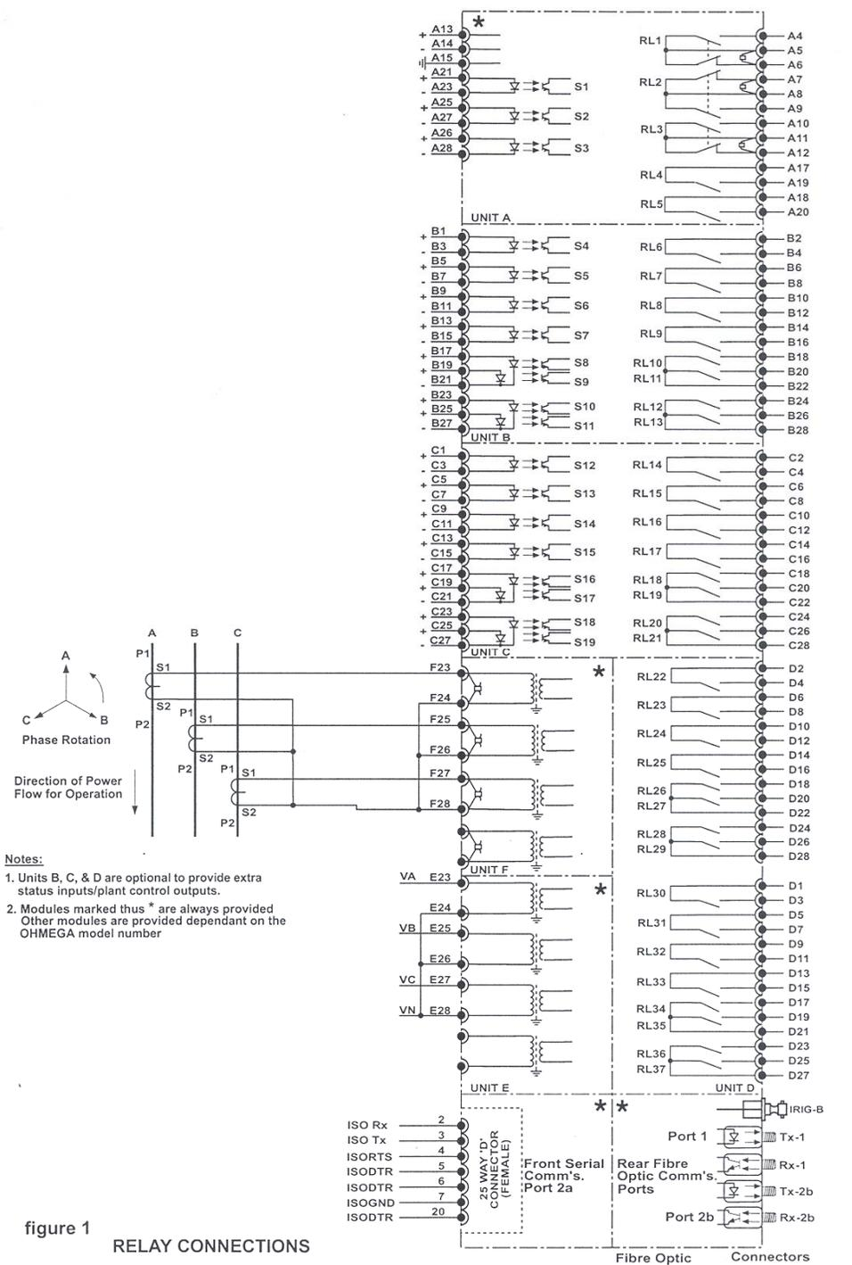
figure 1 RELAY CONNECTIONS
