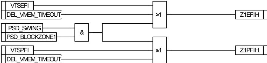
Allow Zone 2 to be inhibited by the same; Power Swing, VTS, or Vmem timed out.
