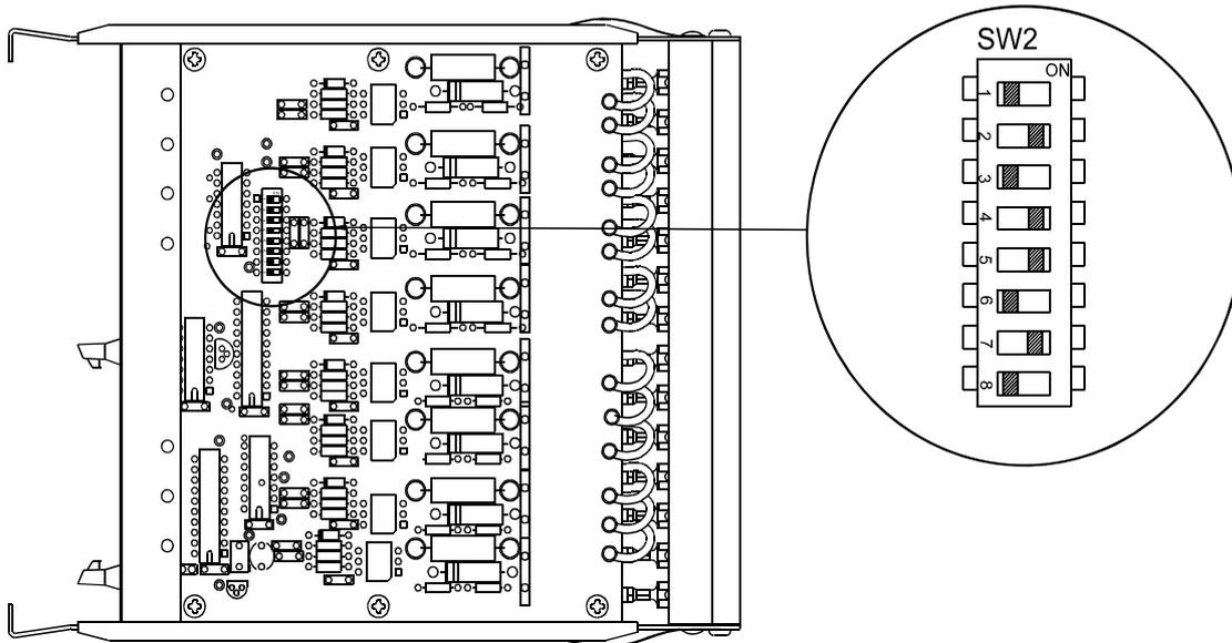
**Note:** Switch SW2 controls 8 status inputs. As supplied, all switches are in the left hand position and all status inputs are high speed devices.
