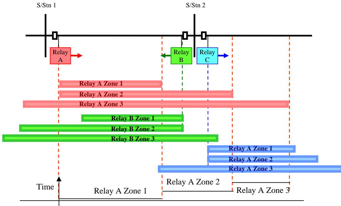
The disadvantage of such a scheme is that faults in the last 20% of the line are cleared after the Zone 2 time delay. This may be acceptable for lower voltage distribution systems, but for important circuits or higher voltage systems additional schemes are available to improve the tripping of the relay.
