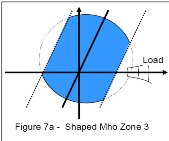
Obviously, this presents no problem for the Quad characteristic, since the reach along the resistive axis can be limited. But the resistive reach of the Mho will depend upon its impedance reach and the degree of offset used.
