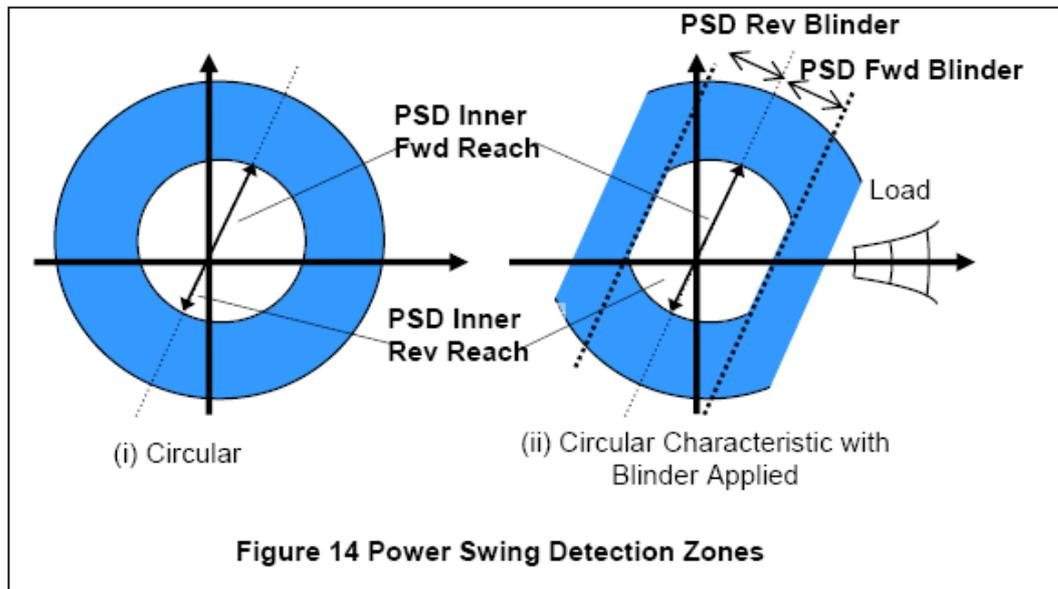
It is possible to apply forward and reverse resistance blinders to the circular characteristic, to separate it from the load impedance if necessary. The user can enable or disable these blinders to achieve the best-tailored shape with reference to load and tripping zones.
