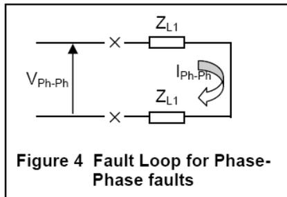
There are three phase fault elements in each zone looking at red-yellow, yellow-blue, and blue-red phase faults respectively. These elements measure the phase-phase voltage, and phase-phase current for their particular phases. As can be seen from figure 4, this leads to a loop impedance of  $2Z_L$ .
