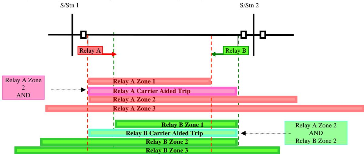
The relay will trip instantaneously for a Zone 1 fault. If a signal is received from the remote end, the time delay will be removed from the Zone 2 element, allowing it to trip instantaneously. The name of the scheme comes from the fact that a Permissive signal is being sent by the Overreaching Zone 2
