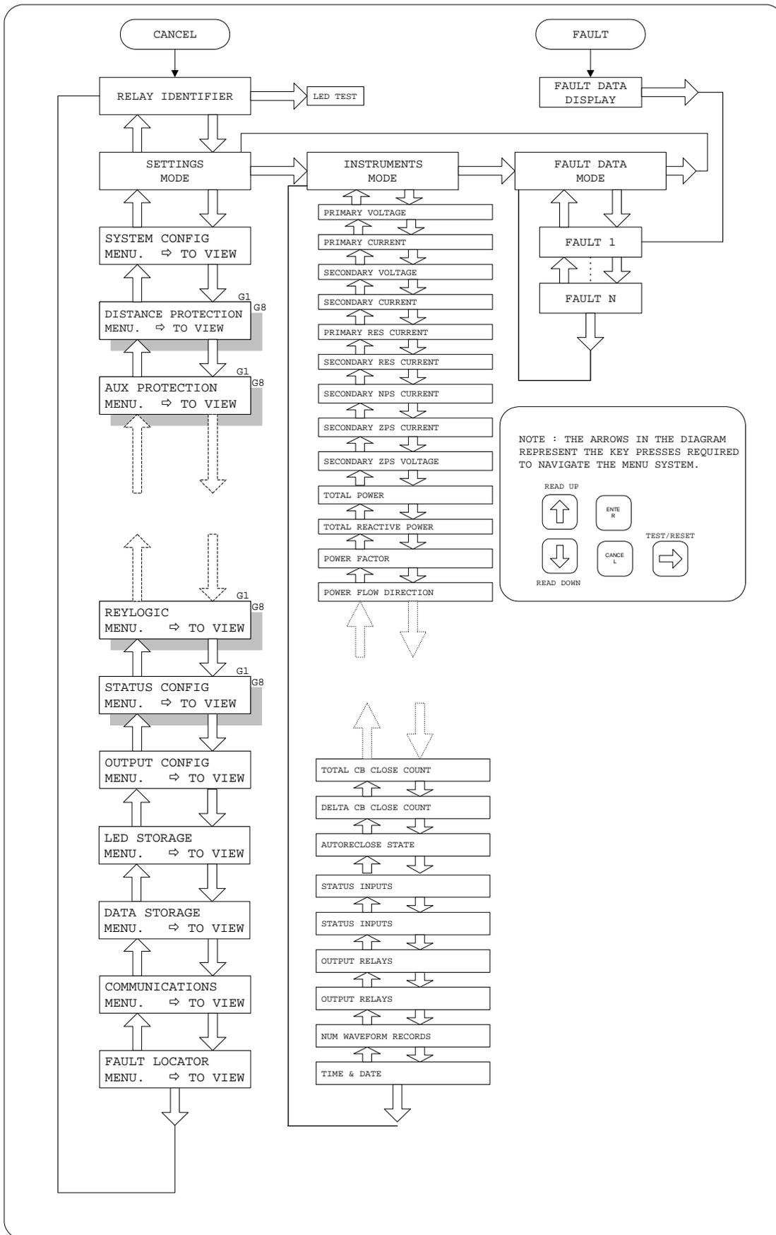
A sub-menu is opened by pressing the ⇨ key when viewing one of the above title screens. The settings within the sub-menu can then be viewed in turn. Leaving a sub-menu, by scrolling either upwards or downwards, causes it to be automatically closed. It must be re-opened in order to view its settings again.
