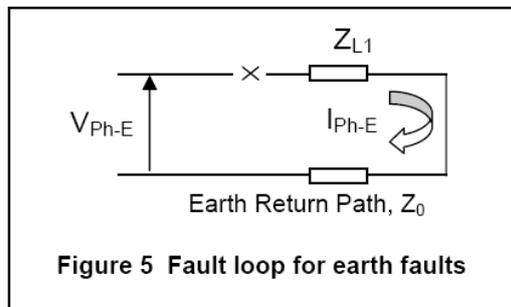
When considering earth faults, the relay is actually presented with a loop impedance of  $Z_L + Z_N$ , where  $Z_L$  is the impedance in the line to the fault and  $Z_N$  is the earth return path, as shown in figure 5. This can also be compensated for by using a combination of the current flowing in the line and neutral circuit but the problem is that the complex impedance  $Z_N$  is not known and is not readily available by measurement.
