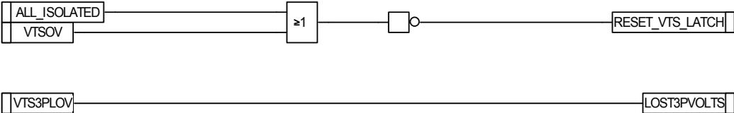
Perform 3 pole loss of voltage check - gives alarm out only.
